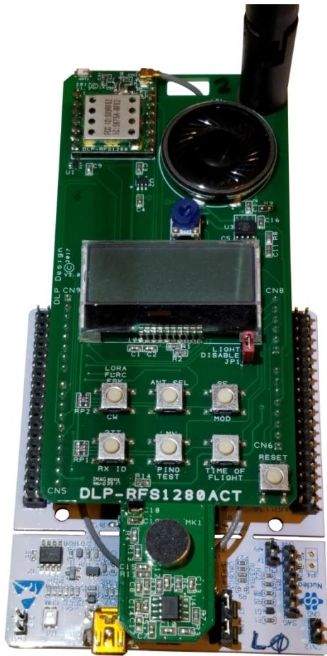
This section describes how to operate the DLP-RFS1280ACT demonstration hardware (purchased separately). The DLP-RFS1280ACT includes a DLP-RFS1280 transceiver module that allows the user to easily verify normal operation of the transceiver and assists in helping them become familiar with the operational firmware.
