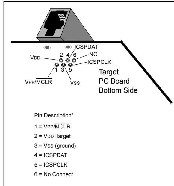
Another connector often found in use with the PICkit™ programmers is a standard 6-pin header with 0.1 inch spacing. Refer to Figure 35-2.
