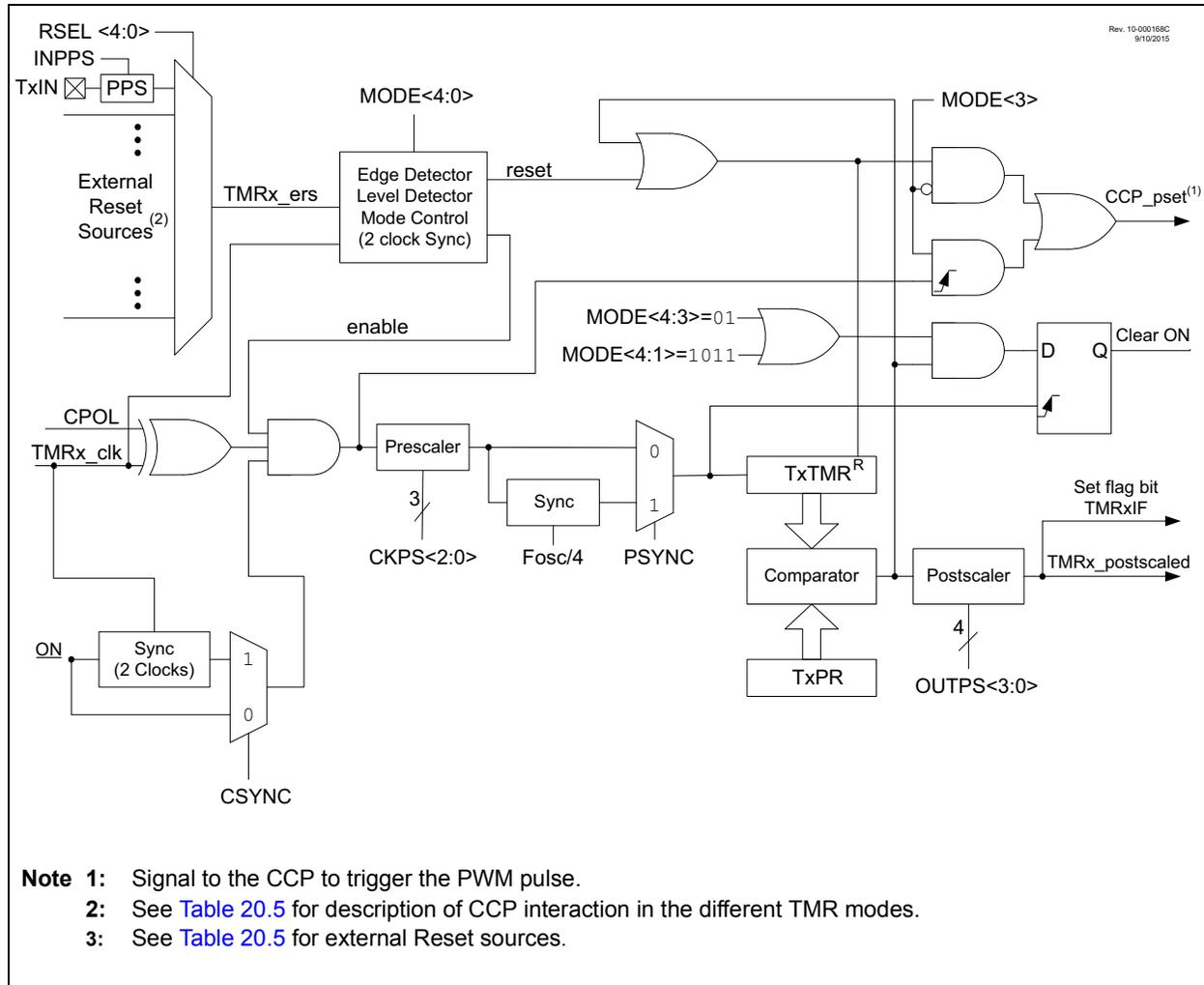
**FIGURE 20-2: TIMER2 CLOCK SOURCE BLOCK DIAGRAM**
