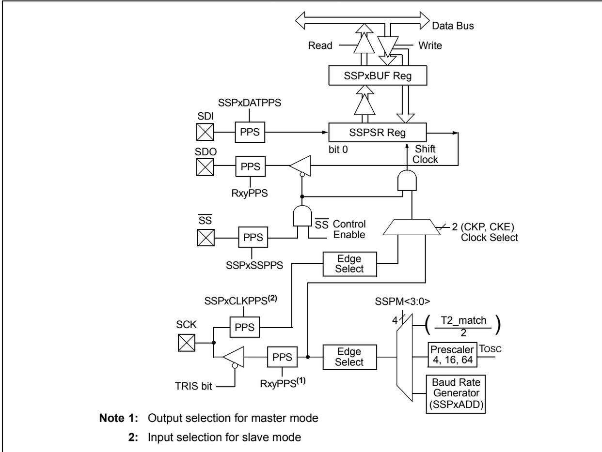
The SPI bus operates with a single master device and one or more slave devices. When multiple slave devices are used, an independent Slave Select connection is required from the master device to each slave device.
