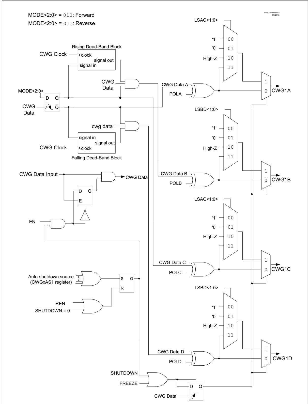
In Forward Full-Bridge mode (MODE<2:0> = 010), CWG1A is driven to its active state, CWG1B and CWG1C are driven to their inactive state, and CWG1D is modulated by the input signal, as shown in Figure 24-7.
