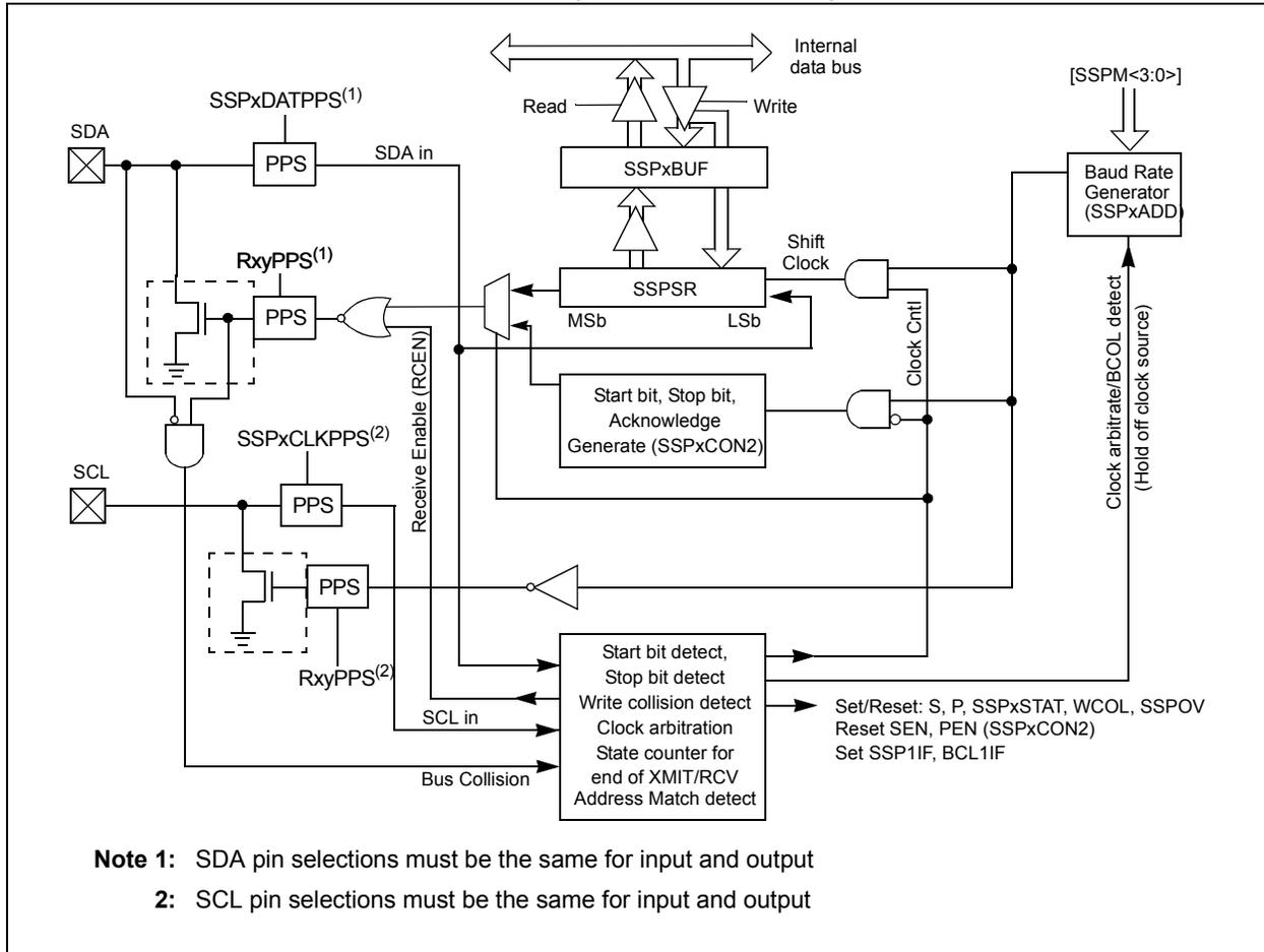
**FIGURE 27-10: MSSP BLOCK DIAGRAM (I<sup>2</sup>C SLAVE MODE)**
