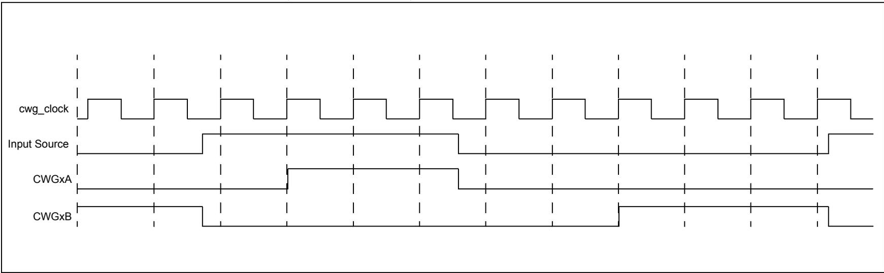
**FIGURE 24-13: DEAD-BAND OPERATION, CWG1DBR = 0x03, CWG1DBF = 0x06, SOURCE SHORTER THAN DEAD BAND**
