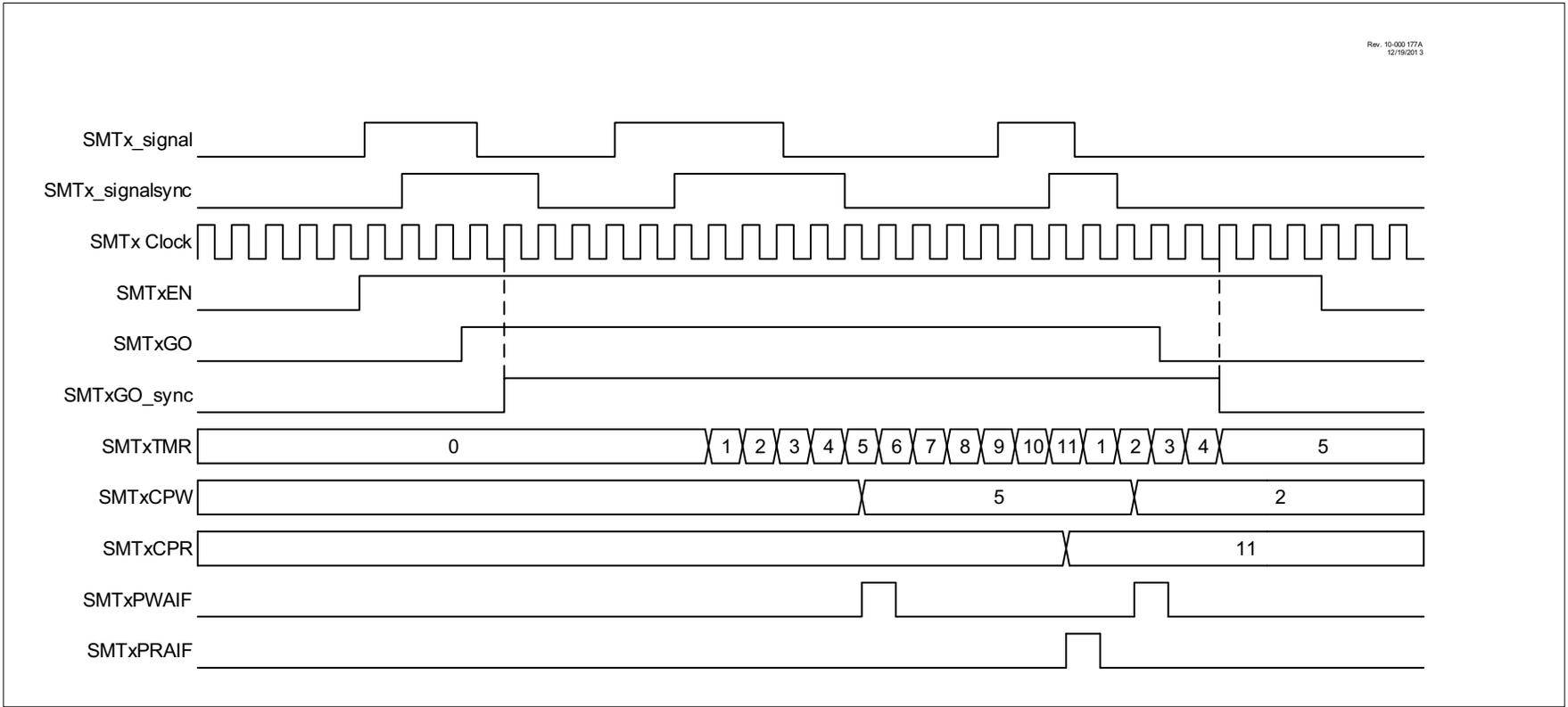
**FIGURE 25-7: PERIOD AND DUTY-CYCLE SINGLE ACQUISITION TIMING DIAGRAM**
