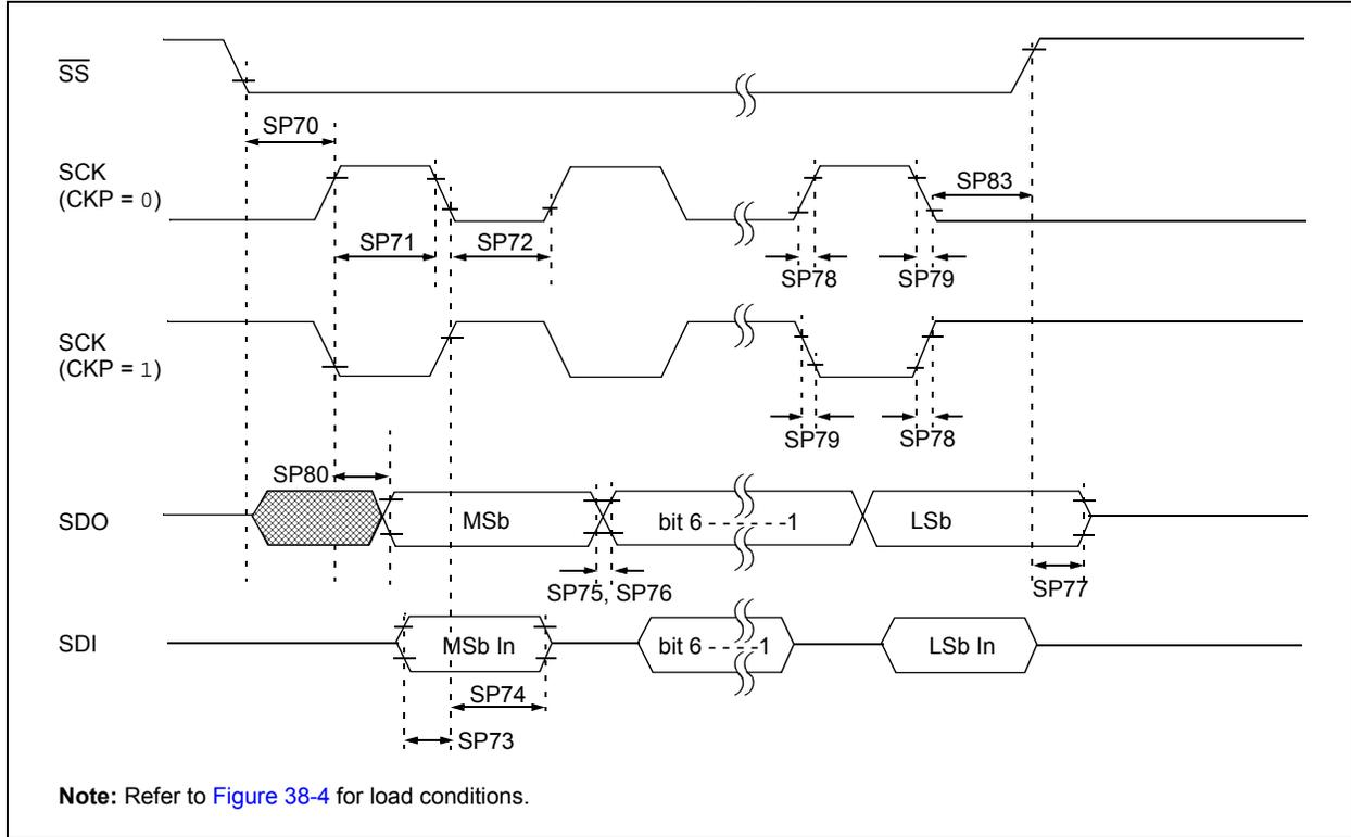
**FIGURE 38-19: SPI SLAVE MODE TIMING (CKE = 1)**
