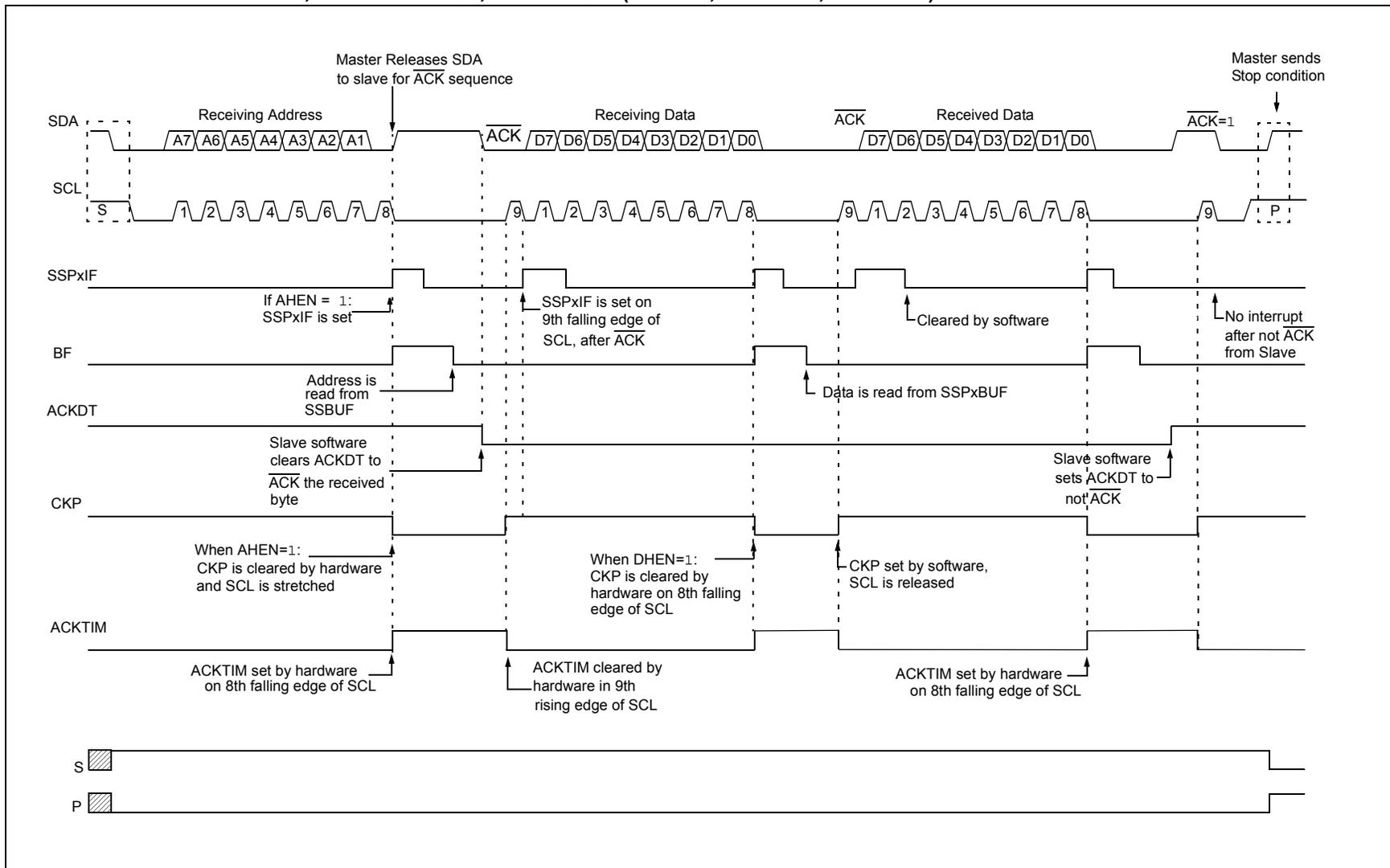
**FIGURE 27-17: I<sup>2</sup>C SLAVE, 7-BIT ADDRESS, RECEPTION (SEN = 1, AHEN = 1, DHEN = 1)**
