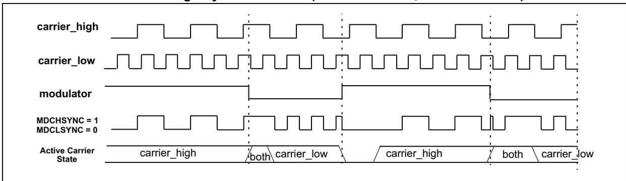
**FIGURE 26-5: Carrier Low Synchronization (MDSHSYNC = 0, MDCLSYNC = 1)**
