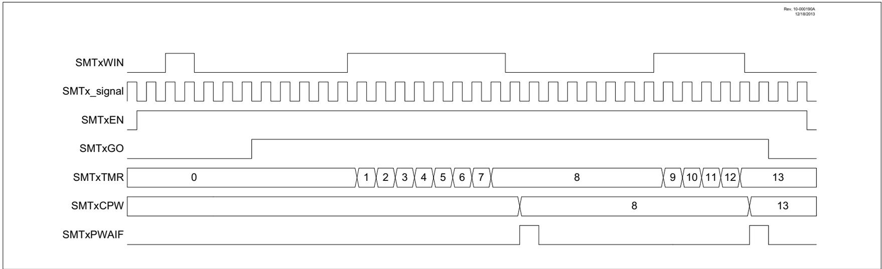
**FIGURE 25-20: GATED COUNTER MODE SINGLE ACQUISITION TIMING DIAGRAM**
