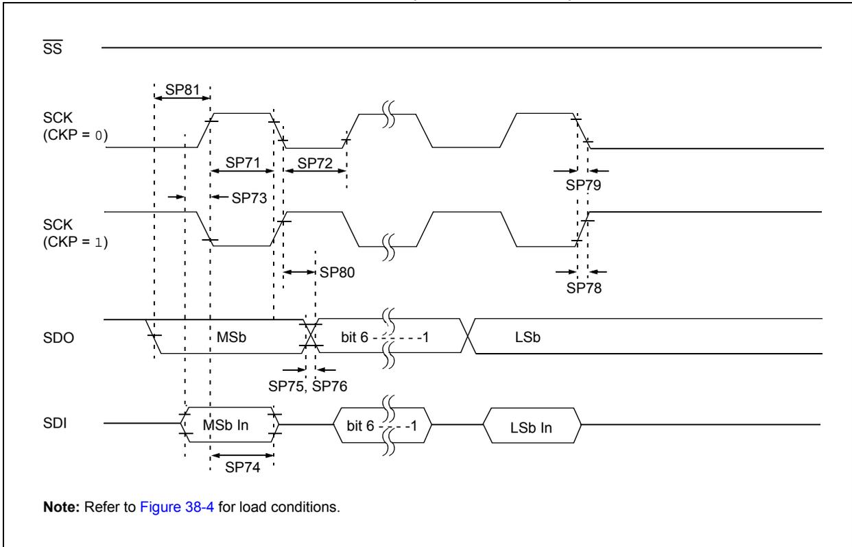
**FIGURE 38-18: SPI SLAVE MODE TIMING (CKE = 0)**
