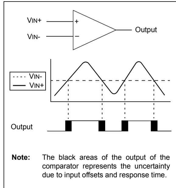
**FIGURE 33-2: COMPARATOR MODULE SIMPLIFIED BLOCK DIAGRAM**
