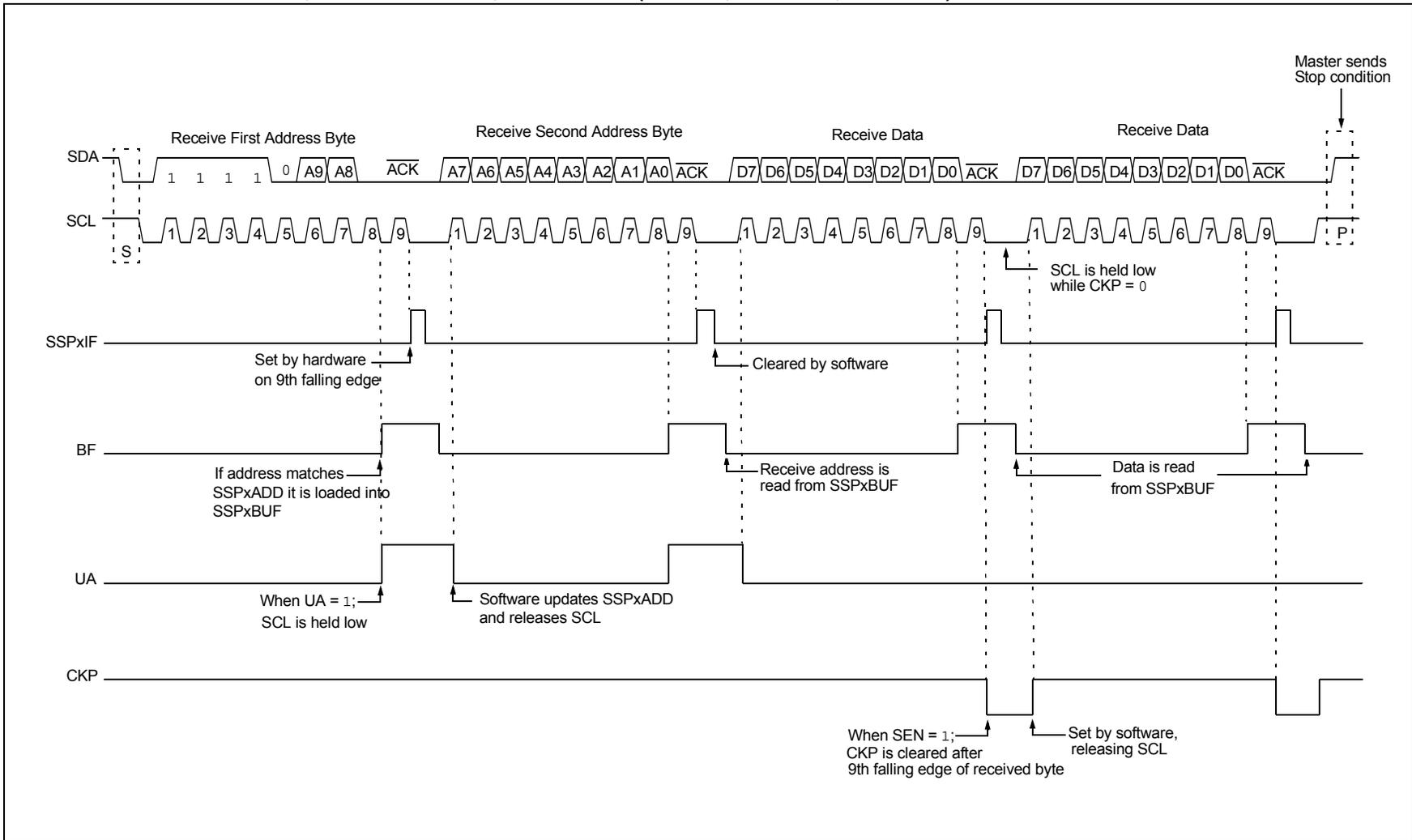
**FIGURE 27-21: I<sup>2</sup>C SLAVE, 10-BIT ADDRESS, RECEPTION (SEN = 0, AHEN = 1, DHEN = 0)**
