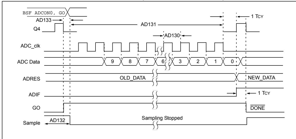
**FIGURE 38-11: ADC CONVERSION TIMING (ADC CLOCK FROM ADCRC)**
