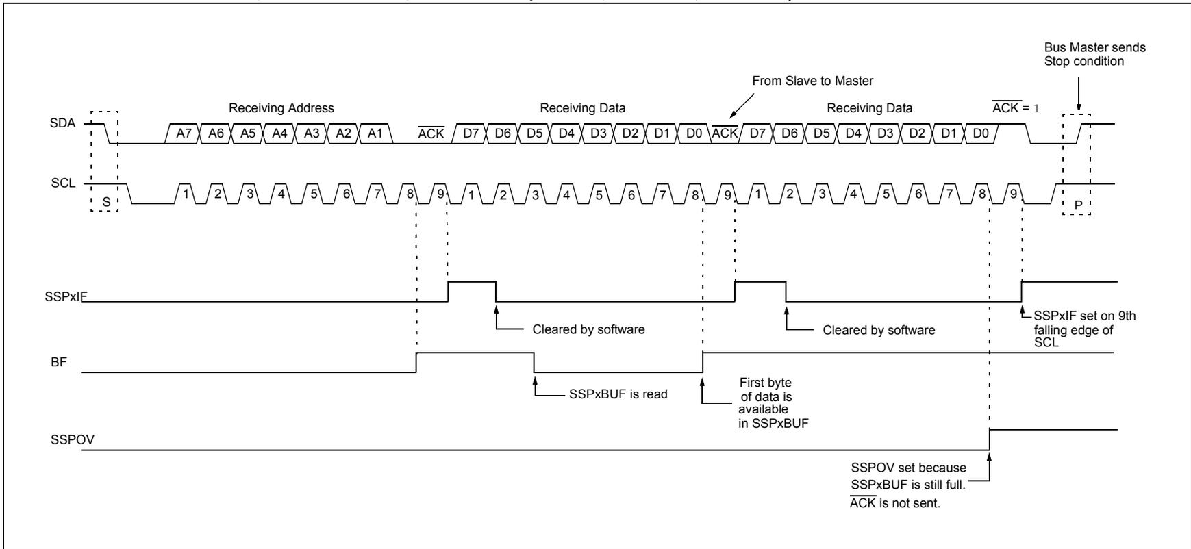
**FIGURE 27-15: I<sup>2</sup>C SLAVE, 7-BIT ADDRESS, RECEPTION (SEN = 1, AHEN = 0, DHEN = 0)**
