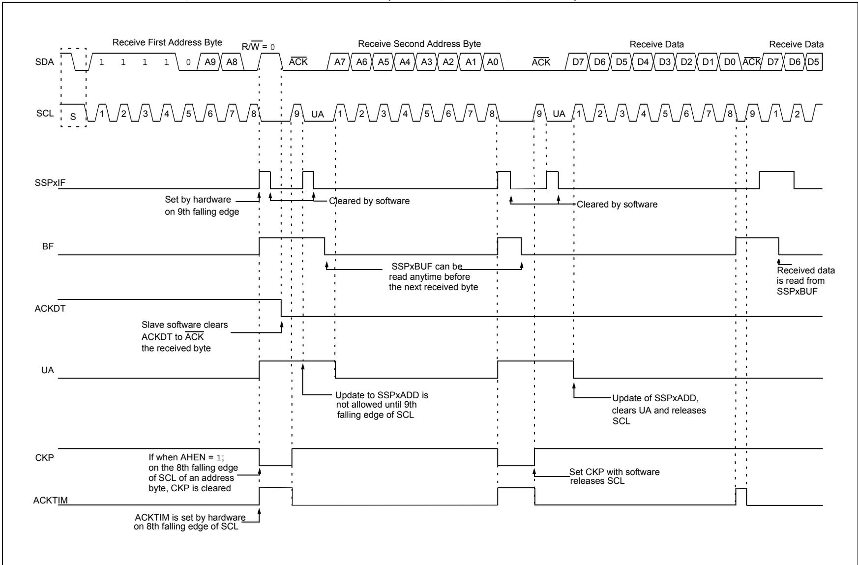
**FIGURE 27-22: I<sup>2</sup>C SLAVE, 10-BIT ADDRESS, TRANSMISSION (SEN = 0, AHEN = 0, DHEN = 0)**
