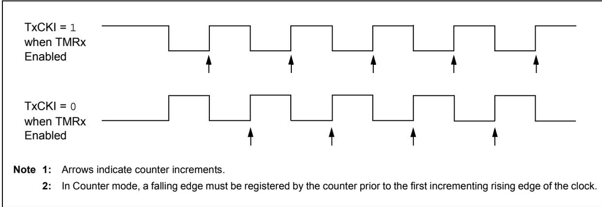
**FIGURE 19-4: TIMER1/3/5/7 GATE ENABLE MODE**
