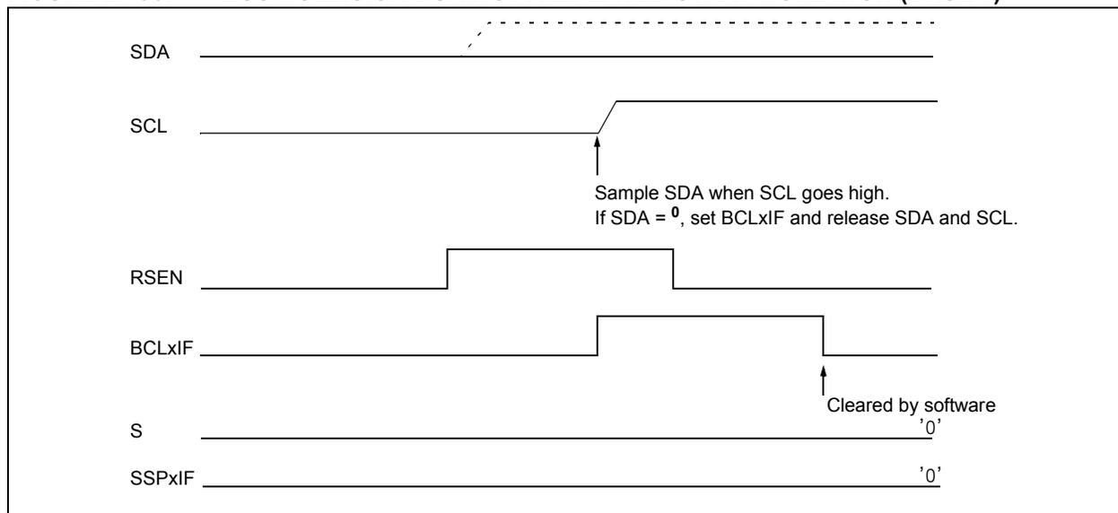
**FIGURE 27-37: BUS COLLISION DURING REPEATED START CONDITION (CASE 2)**
