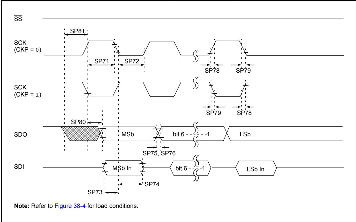
**FIGURE 38-17: SPI MASTER MODE TIMING (CKE = 1, SMP = 1)**
