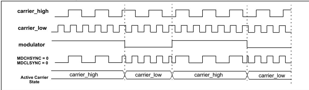
**FIGURE 26-4: Carrier High Synchronization (MDSHSYNC = 1, MDCLSYNC = 0)**
