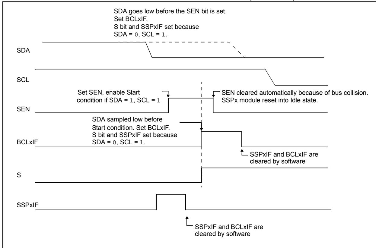
**FIGURE 27-34: BUS COLLISION DURING START CONDITION (SCL = 0)**
