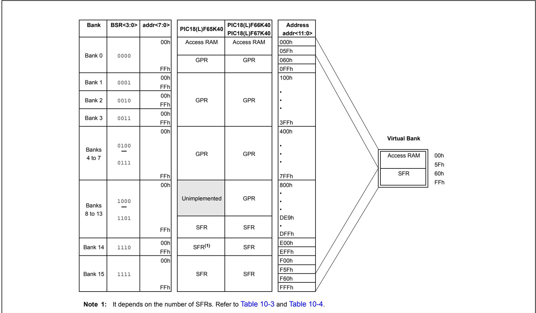
**FIGURE 10-5: USE OF THE BANK SELECT REGISTER (DIRECT ADDRESSING)**
