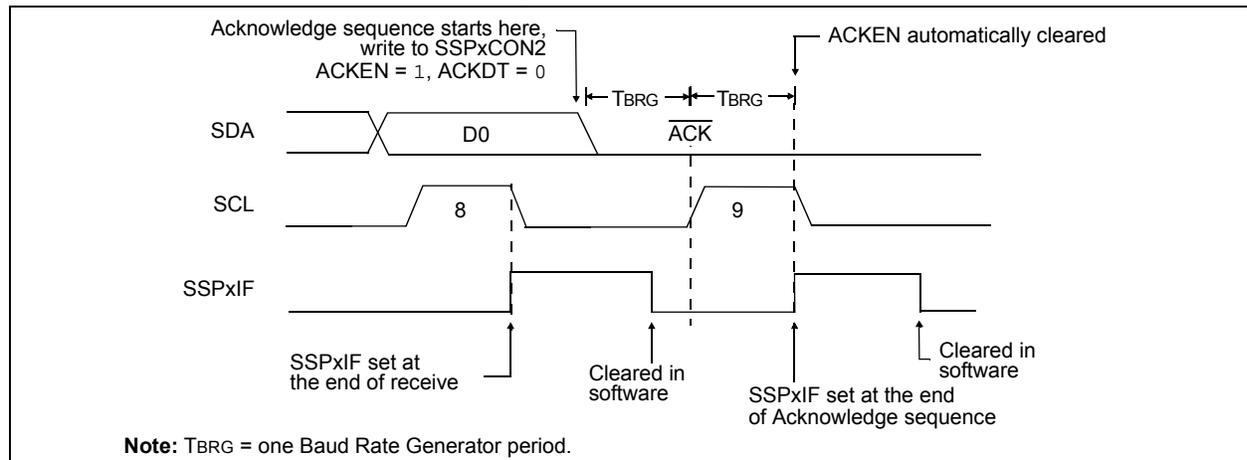
**FIGURE 27-31: STOP CONDITION RECEIVE OR TRANSMIT MODE**
