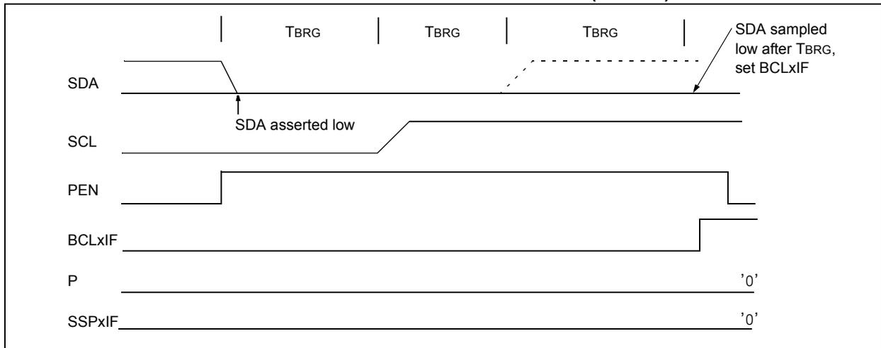
**FIGURE 27-39: BUS COLLISION DURING A STOP CONDITION (CASE 2)**
