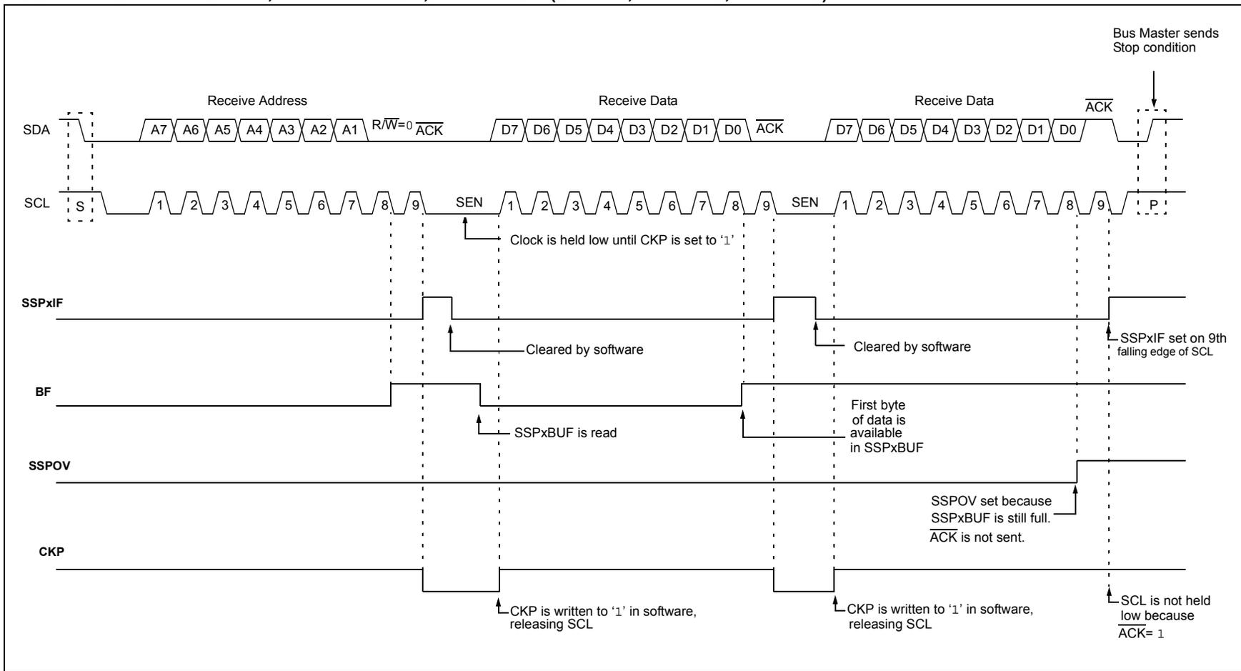
**FIGURE 27-16: I<sup>2</sup>C SLAVE, 7-BIT ADDRESS, RECEPTION (SEN = 0, AHEN = 1, DHEN = 1)**
