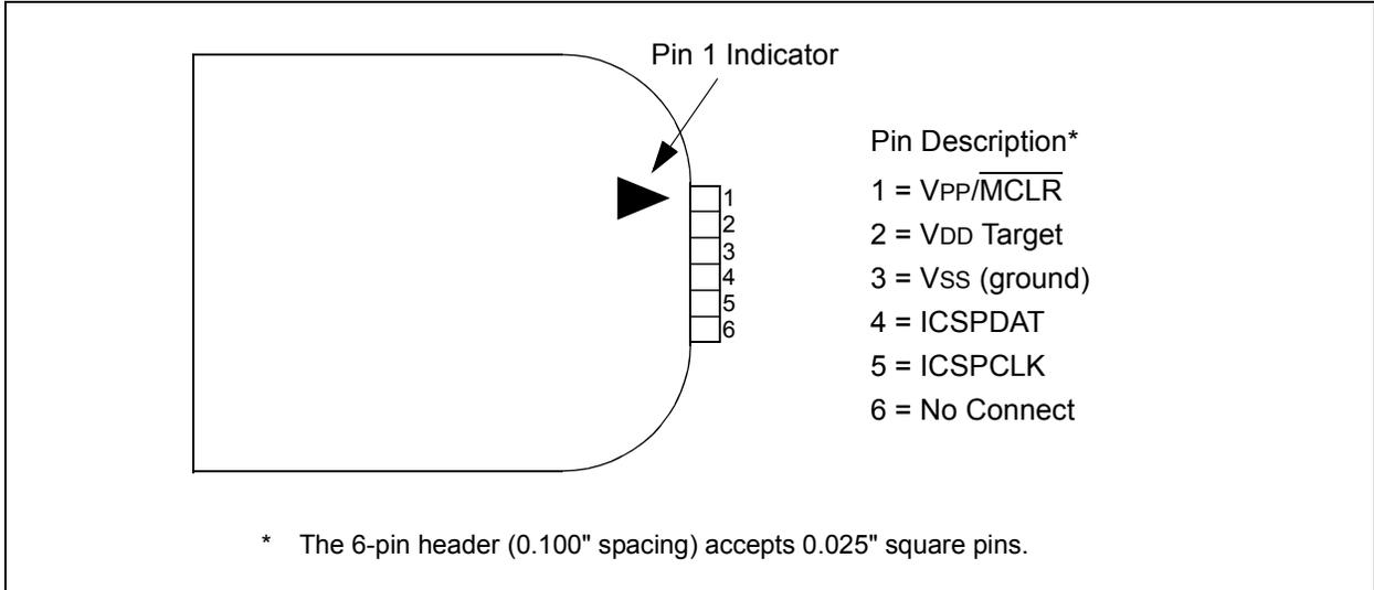
**FIGURE 35-3: TYPICAL CONNECTION FOR ICSP™ PROGRAMMING**
