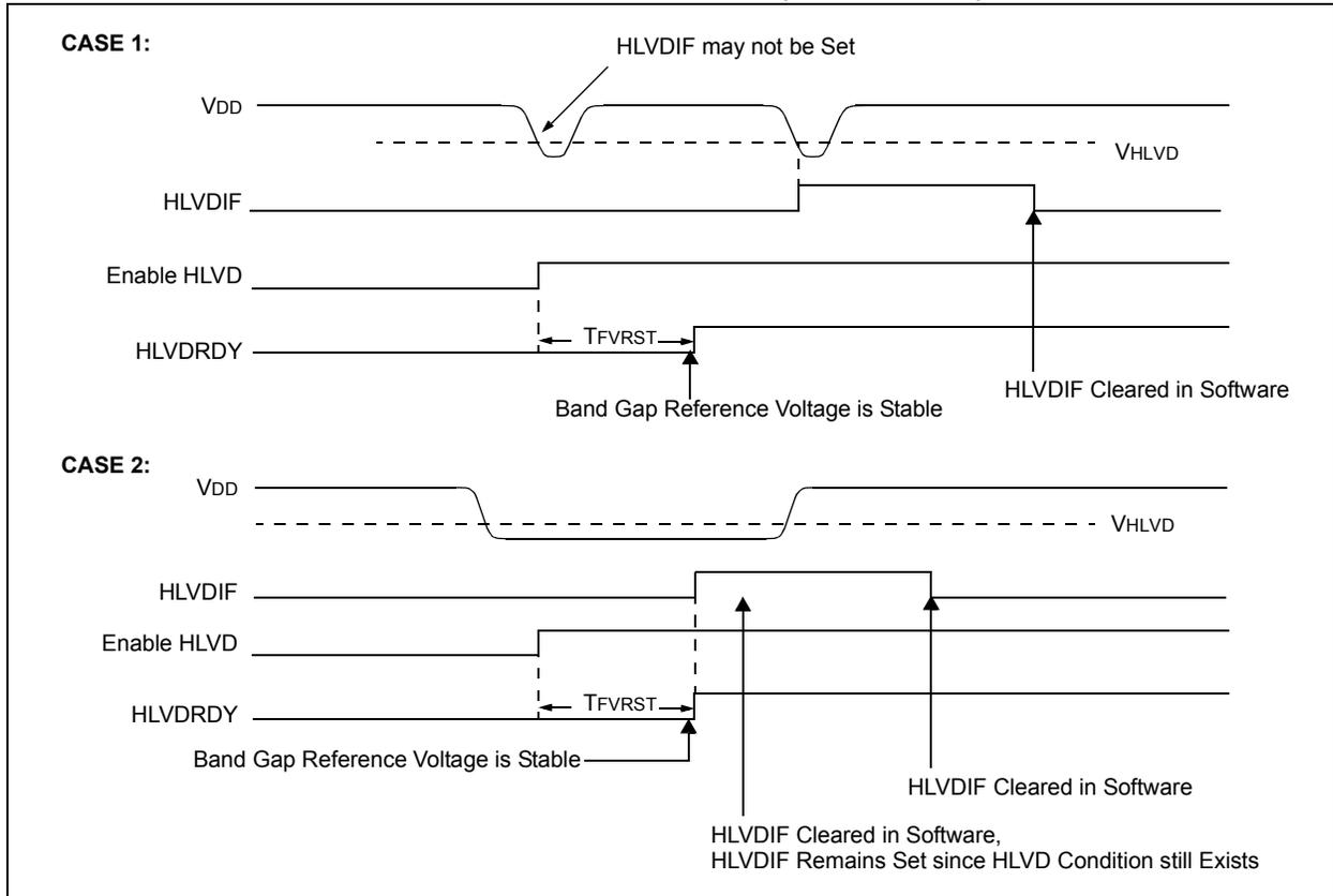
**FIGURE 34-3: HIGH-VOLTAGE DETECT OPERATION (HLVDINTH = 1)**
