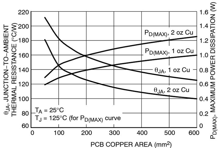
Figure 30.  $\theta_{JA}$  and  $P_{D(MAX)}$  vs. Copper Area
