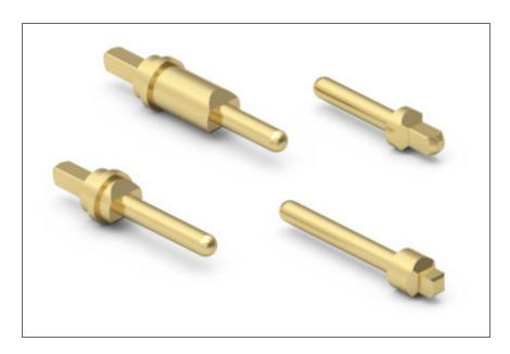
Mill-Max Manufacturing Corp., Inc. today announces four new pins specifically designed for press-fit into PCB plated-through holes, providing a secure connection while maintaining plated-through hole integrity and continuity. These new PCB pins incorporate square press-fit geometry and angled vent features making them suitable for solderless press-fit or press-fit and solder PCB termination.
